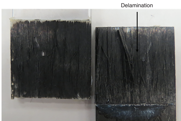
Figure 1.36 Example of delamination failure of composite joints.
