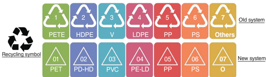
Figure 1.2 Comparison of the familiar SPI system and the new ASTM system for plastic identification. Source: Crawford and Quinn [2]. Copyright 2017. Reproduced with permission from Elsevier.
