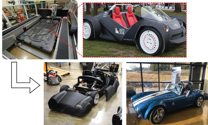
Figure 1.11 Cincinnati Inc.'s BAAM system in collaboration with ORNL (build volume of 1829 \times 3658 \times 914 mm ( 6 \times 12 \times 3 ft)) printing Local Motors's Strati. The system was used to build a Shelby Cobra replica. Source: Oak Ridge National Laboratory / Public Domain.
