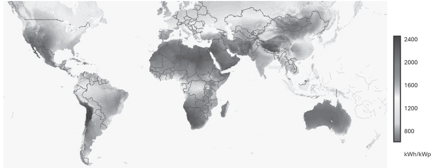
Figure 1.3 Solar irradiance over the world in kWh/day/m 2 (Global Solar Atlas [21]; map from Global Solar Atlas 2.0, Global Solar Atlas).
