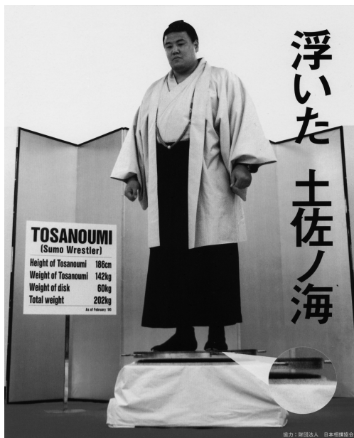
Fig. 1.4 Application of free levitation by means of the permanent currents in a superconductor. The Sumo wrestler (including the plate at the bottom) weighs 202 kg. The superconductor is \text{YBa}_2\text{Cu}_3\text{O}_7 . (Photograph kindly supplied by the International Superconductivity Research Center (ISTEC) and Nihon-SUMO Kyokai, Japan, 1997).
