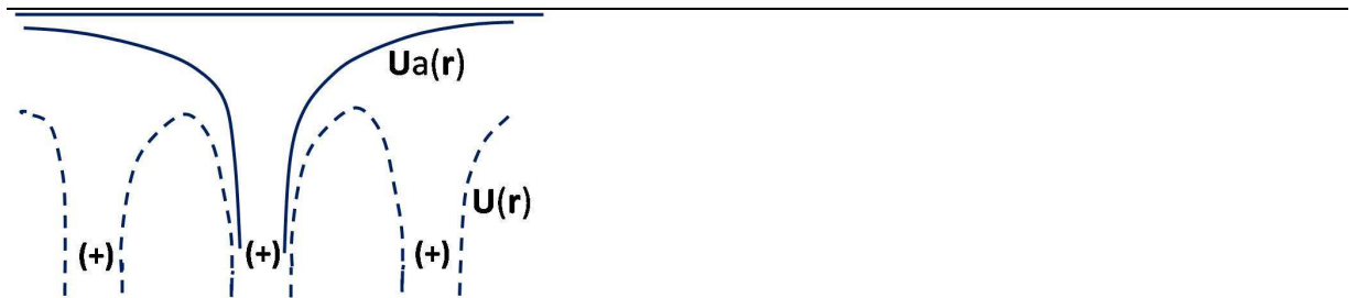
Figure 4.5: Comparison of the potential energy of an electron in the case of a single individual atom, U_a(\mathbf{r}) (solid curve), and in the presence of atoms at the neighboring lattice sites, U(\mathbf{r}) (dashed curve).
