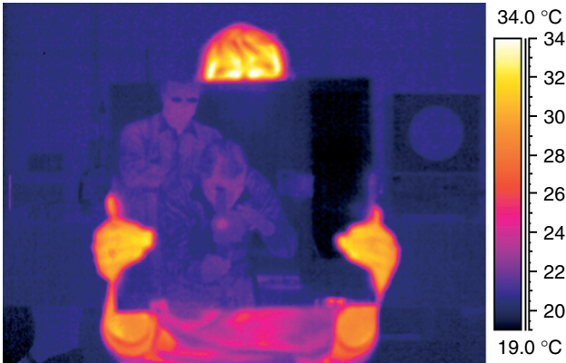
Figure 5.38 A room temperature glass plate is opaque to IR radiation. In addition, due to the flat surface, it serves as a source of thermal reflections, here two people standing behind the IR camera.
