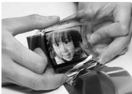
Figure 1.92 A flexible, full-color organic electroluminescent display (OLED) built using organic thin-film transistor (TFT) technology with a plastic substrate. The 2.5 in prototype display, which is 0.3 mm thick and weighs 1.5 g without the driver, supports 16.8 million colors at
