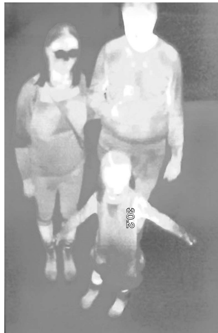
Figure 1.2 Example of an infrared image from a thermal imager. The skin has the highest temperature and hence the highest emission.
