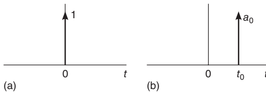
Figure 1.9 (a) Usual representations of the impulse function \delta(t) and (b) the shifted (and escalated) impulse function a_0 \delta(t - t_0) .
