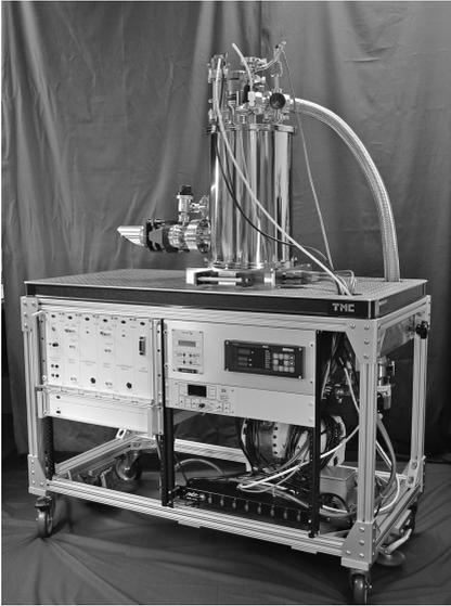
**Fig. 1-22** A cryogenic radiometer as used for characterization of flight pyrheliometers and spectra-radiometers, constructed by L-1 Standards, Inc., under licence from Cambridge Research and Instrumentation, Inc. Intensity-stabilized, polarized, laser light is introduced into the cryo-radiometer cavity through a Brewster-angled window in the horizontal snout. The same laser beam is used to illuminate the flight radiometer. By permission of Steven Lorenz, L-1 Standards, Inc.
