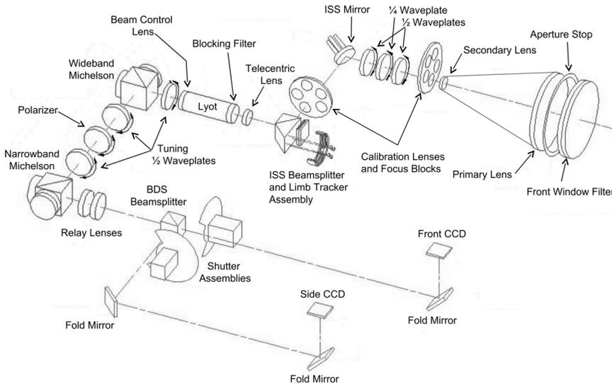
**Fig. 1-20** Optical layout of the Helioseismic Magnetic Imager (HMI) showing the imaging optics, polarization analyzers, Lyot and Michelson monochromators, and detectors. By permission of J. Schou, Stanford University.
