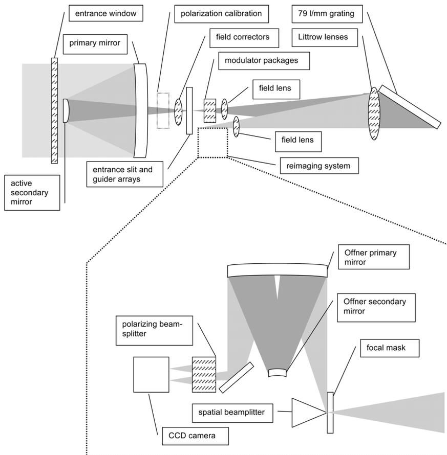
**Fig. 1-23** Optical layout of the SOLIS synoptic telescope at the U.S. National Solar Observatory, Kitt Peak, Arizona. Kindly provided by L. Bertello.
