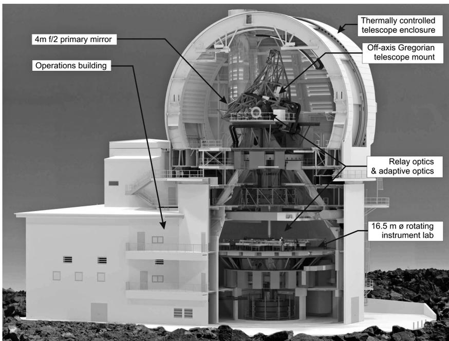
**Fig. 1-18** A design for the proposed 4-meter class Advanced Technology Solar Telescope, making use of adaptive optics to achieve angular resolution better than 50 milli-arc secs. The ATST is optimized for wavelength coverage extending beyond 20 microns in the infra-red, and low instrumental polarization. Figure kindly provided by the U.S. National Solar Observatory.
