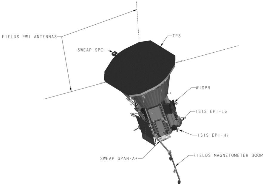
**Fig. 1-19** Artist's impression of the Solar Probe Plus showing the thermal protection system (TPS), the imager (WISPR), the solar particle experiments (SWEAP, SPC, SPA), and the fields detection antennas and boom. The imaging instrument will operate in the penumbra of the heat shield, where moderate temperatures are expected. By courtesy of NASA.
