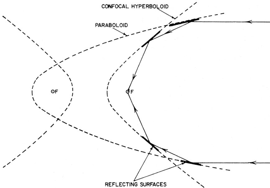
**Fig. 1-17** The principle of a soft X-ray imaging telescope. Light entering from the right is reflected at grazing incidence from surfaces of confocal hyperboloid and paraboloid mirrors and is brought to the focus at F. Film is usually used as a detector. By permission of L. Golub.
