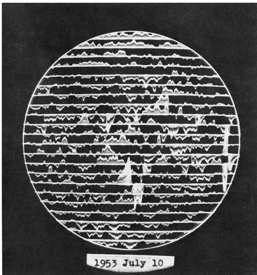
**Fig. 1-14** An early photoelectric magnetogram obtained with the Babcock magnetograph. Each trace was made by a separate scan across the sun. A deflection equal to the distance between traces is produced by a field (averaged over the spectrograph entrance slit) of about 10 G. By permission of the University of Chicago Press.
