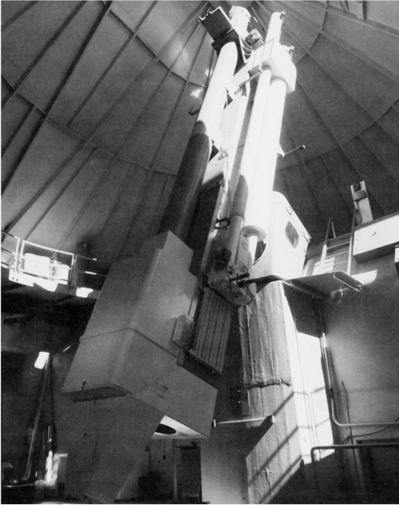
**Fig. 1-16** The 16-inch aperture coronagraph at Sacramento Peak Observatory in New Mexico. This instrument is in active use for coronal studies and other observations requiring low scattered light. National Solar Observatories photograph.
