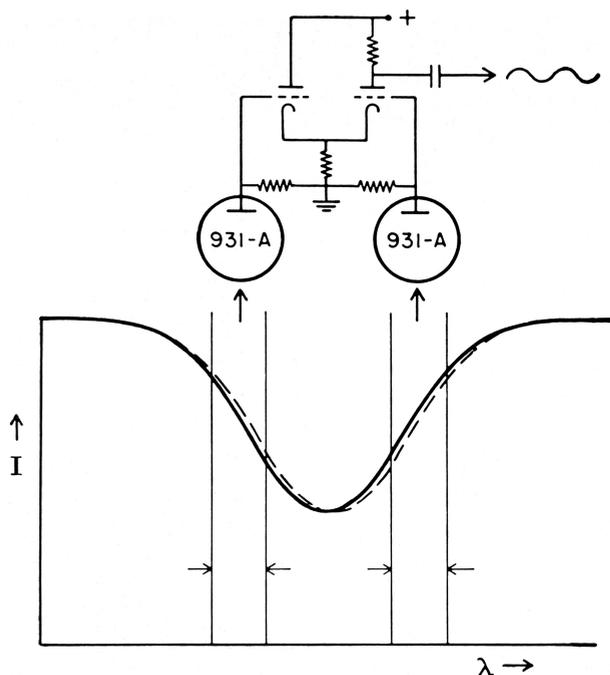
**Fig. 1-13** Schematic diagram showing the principle of operation of the original Babcock magnetograph. Profiles of an absorption line for the two states of opposite circular polarization are shown solid and dashed. The symbols  $I$  and  $\lambda$  refer to intensity and wavelength respectively. The two detectors are type 931-A photomultipliers. By permission of the University of Chicago Press.
