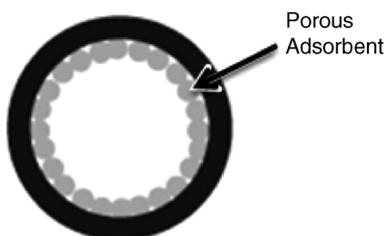
**Figure 3.2** Porous layer open tubular column ( <http://community.asdlib.org/imageandvideoexchange/2011/06/21/gc-columns/>).
