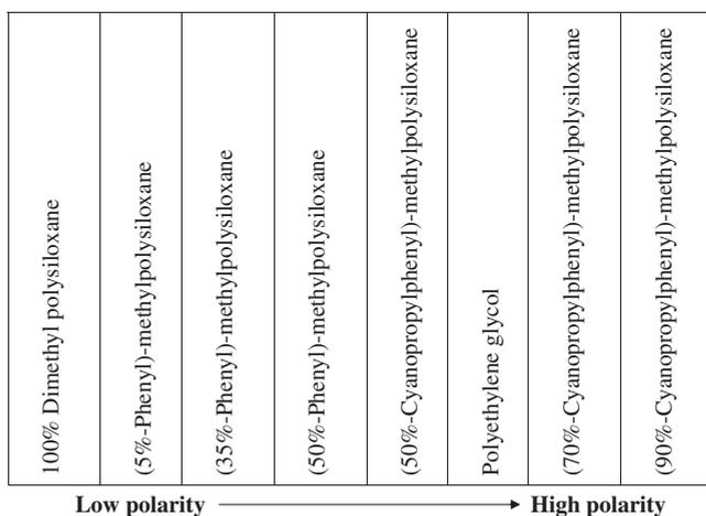
**Figure 3.6** Classification of GC stationary phases with regard to polarity. (Reproduced with permission from Ref. [14].)
