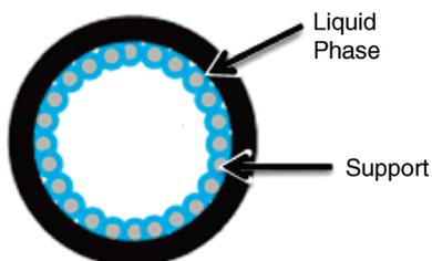
**Figure 3.4** Support-coated open tubular column ( <http://community.asdlib.org/imageandvideoexchangeforum/2011/06/21/gc-columns/>).
