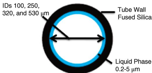
**Figure 3.3** Wall-coated open tubular (WCOT) column ( <http://community.asdlib.org/imageandvideoexchangeforum/2011/06/21/gc-columns/>).
