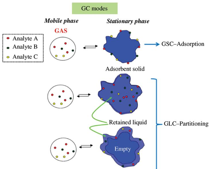
**Figure 3.1** GC modes showing interaction between the mobile phase and the stationary phases.
