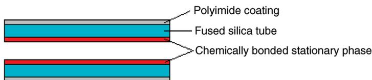
**Figure 3.5** Cross-section of a fused silica open tubular column (<http://teaching.shu.ac.uk/hwb/chemistry/tutorials/chrom/gaschrom.htm>).
