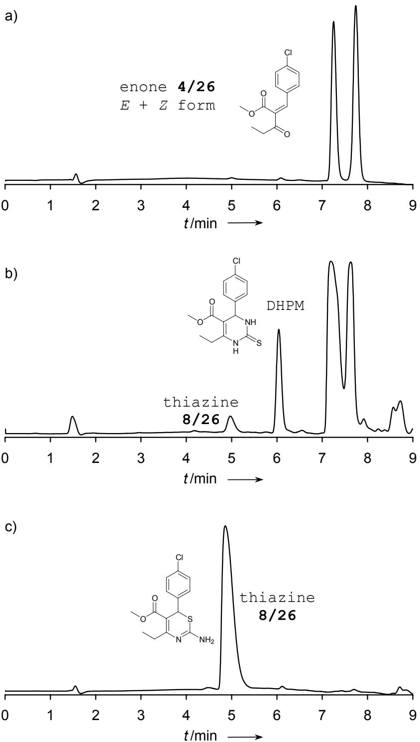
Analytical HPLC of thiazine synthesis. a) after Knoevenagel condensation (*E/Z* isomers); b) wash step, traces of product **8/26** at  $t = 5\text{min}$ , dihydropyrimidinethione (DHPM) byproduct at  $t = 6\text{ min}$ ; c) final product **8/26** after resin release.
