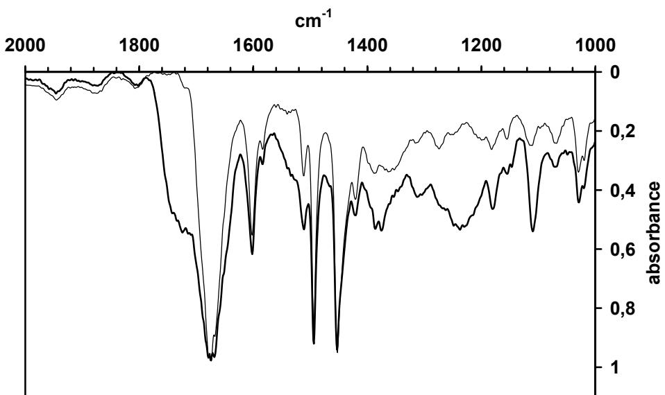
On-bead FT-IR analysis of the reaction of diisopropyl azodicarboxylate (DIAD) with scavenger resin **11**. Thin line: resin **11**; thick line: **11** after reaction with DIAD. The carbonyl groups at ca 1700-1710 cm<sup>-1</sup> reflect the ester bonds in **13** or **14**.
