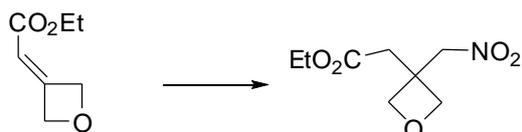
To a solution of  $\alpha,\beta$ -unsaturated ester **25** (1.62 g, 11.4 mmol, 1.00 equiv) in 10 mL dry MeCN was added nitro methane (3.08 mL, 56.9 mmol, 5.00 equiv), followed by a catalytic amount of DBU (340  $\mu$ L, 2.28 mmol, 0.200 equiv) at 0°C. After stirring for 4h at rt, the mixture was filtered through a plug of SiO<sub>2</sub> with 4/1 cyclohexane/EtOAc to give 2.13 g almost (>98 w% by NMR) pure material as a colorless liquid (92 % yield).
