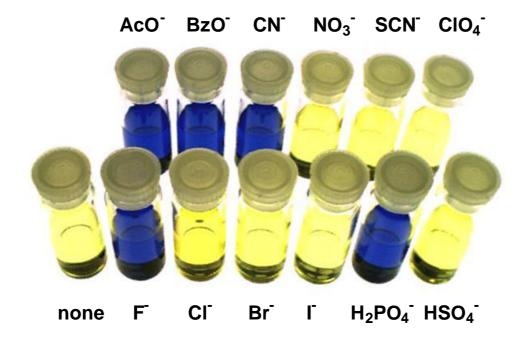
Alizarin in dichloromethane (1 x  $10^{-4}$  M). The color changed from yellow to blue by F<sup>-</sup>, H<sub>2</sub>PO<sub>4</sub><sup>-</sup>, AcO<sup>-</sup>, BzO<sup>-</sup> and CN<sup>-</sup> (Anion: 100 equiv.).
