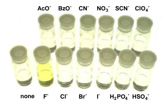
L-leucine-4-nitroanilide in dichloromethane (1 x  $10^{-4}$  M). The color changed from colorless to intense yellow by  $F^-$ , to weak yellow by  $CN^-$  (Anion: 100 equiv.).
