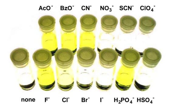
4-nitrophenol in dichloromethane (1 x  $10^{-4}$  M). The color changed from colorless to intense yellow by F<sup>-</sup>,  $H_2PO_4^-$ , AcO<sup>-</sup>, BzO<sup>-</sup> and CN<sup>-</sup>, to yellow by Cl<sup>-</sup> (Anion: 100 equiv.).
