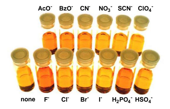
1,8-diaminoanthraquinone in dichloromethane (1 x  $10^{-4}$  M). The color changed from orange to reddish orange by F<sup>-</sup>,  $H_2PO_4^-$ , AcO<sup>-</sup>, BzO<sup>-</sup> and CN<sup>-</sup> (Anion: 100 equiv.).
