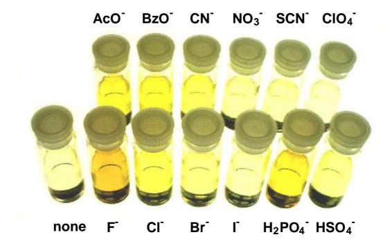
4-nitro-1,2-phenylenediamine in dichloromethane (1 x  $10^{-4}\,\mathrm{M}$ ). The color changed from pale yellow to orange by F<sup>-</sup>, to intence yellow by Cl<sup>-</sup>,  $\mathrm{H_2PO_4}^-$ , AcO<sup>-</sup>, BzO<sup>-</sup> and CN<sup>-</sup>, to yellow by Br<sup>-</sup>,  $\mathrm{HSO_4}^-$ ,  $\mathrm{NO_3}^-$  and SCN<sup>-</sup> (Anion: 100 equiv.).
