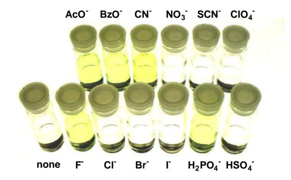
Naphthol AS in dichloromethane (1 x  $10^{-4}$  M). The color changed from colorless to fluorescent yellow by F<sup>-</sup>, H<sub>2</sub>PO<sub>4</sub><sup>-</sup>, AcO<sup>-</sup>, BzO<sup>-</sup> and CN<sup>-</sup> (Anion: 100 equiv.).
