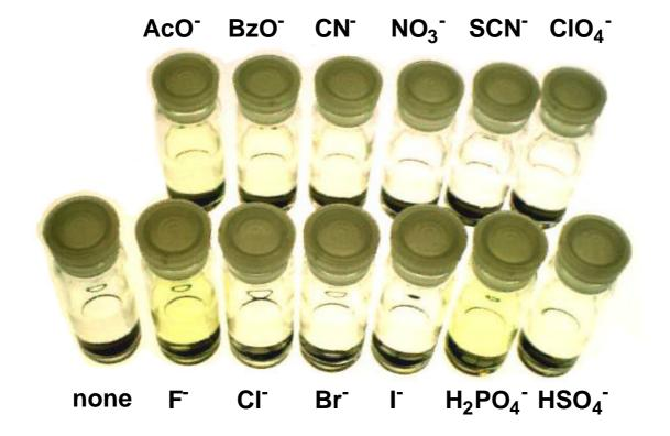
4-nitroaniline in dichloromethane (1 x  $10^{-4}$  M). The color changed from colorless to yellow by F<sup>-</sup>, H<sub>2</sub>PO<sub>4</sub><sup>-</sup>, AcO<sup>-</sup>, BzO<sup>-</sup> and CN<sup>-</sup> (Anion: 100 equiv.).
