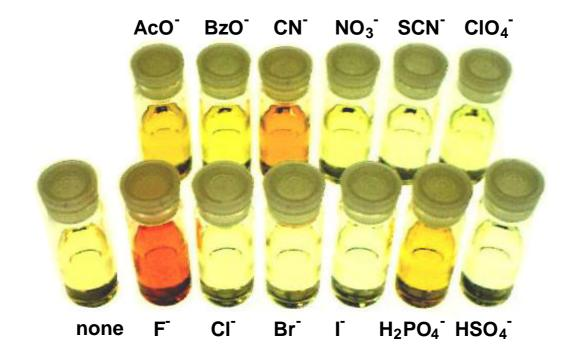
$1\text{-}(4\text{-nitrophenyl})\text{-}2\text{-thiourea in DMSO }(1\text{ x }10^{-4}\text{ M})\text{.} \quad \text{The }$  color changed from pale yellow to orange by \$F^-\$ and \$CN^-\$, to intense yellow by \$H\_2PO\_4^-\$, \$AcO^-\$ and \$BzO^-\$ (Anion: 100 equiv.).}
