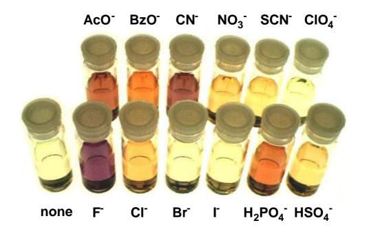
2,2'-bi(3-hydroxy-1,4-naphthoquinone) in dichloromethane (1 x  $10^{-4}$  M). The color changed from yellow to purple by F<sup>-</sup>, CN<sup>-</sup>, to reddish orange by  $H_2PO_4^-$ , AcO<sup>-</sup> BnO<sup>-</sup>, to yellow by Cl<sup>-</sup>,  $HSO_4^-$ ,  $NO_3^-$  and  $SCN^-$  (Anion: 100 equiv.).
