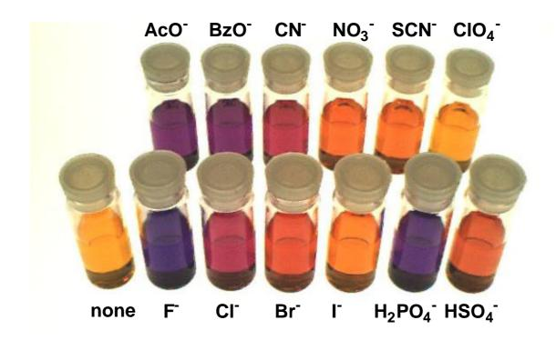
1,2-diaminoanthraquinone in dichloromethane (1 x  $10^{-4}$  M). The color changed from yellow to dark purple by  $F^-$ , to red by  $Cl^-$ , to reddish orange by  $Br^-$ , to orange by  $I^-$ , to purple by  $H_2PO_4^-$ , to orange by  $HSO_4^-$ , to purple by  $AcO^-$  and  $BzO^-$ , to red by  $CN^-$ , to orange by  $NO_3^-$ , to orange by  $SCN^-$  (Anion: 100 equiv.).
