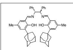
diphenylethylenediamine (1f). IR (neat): 3440 (br, m), 2910 (s), 1630 (s) cm $^{-1}$ ;  $^{1}$ H NMR:  $\delta$ 13.43 (2 H, s, OH), 8.27 (2 H, s, ArCHN), 7.17 (10 H, m, aromatic), 6.95 (2 H, d, J=2.0 Hz, phenyl), 6.72 (2 H, d, J=2.0 Hz, phenyl), 4.65 (2 H, s, NCHPh), 1.76-2.14 (36 H, m, alkyl);  $^{13}$ C
