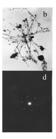
TEM images of the as-synthesized metallic nanowires via the vacuum-pyrolysis-carbothermal route. (a), (b) and (c) correspond to the nanowires of Cd, Cu and Co. (d) is the SAED pattern taken on an individual Co nanowires in (c).
