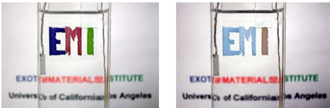
Fig. S8: A device made by using initials of “Exotic Materials Institute” using PEDOT as blue, P3MT as red and PDDTP as green color. Polymer films switch from RGB colors in their neutral state to transmissive colors in their oxidized state.
