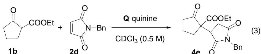
Order in ethyl 2-oxocyclopentane carboxylate **1b** was established by using a large excess of *N*-benzylmaleimide **2d** (5 equiv) and 10 mol% **Q**. Plotting in  $\ln[\mathbf{1b}]$  versus time gave a straight line ( $R^2 = 0.9993$ , Figure 8), thus establishing a first-order dependence on **1b**.
