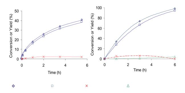
Figure S1: Evolution of species with time during the hydrogenation of nitrobenzene (a), and nitrostyrene (b).
