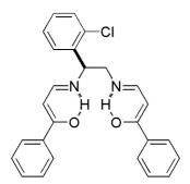
ethylenediamine (3e). Following General Procedure A, from (1*S*)-o-chlorophenyl-1,2-ethylenediamine (218 mg, 1.28 mmol) and benzoylacetaldehyde (379 mg, 2.56 mmol), after stirring at 50 °C for 14 h, was obtained **3e**. The product was purified by silica gel column chromatography (25 $\rightarrow$ 50% EtOAc in hexanes) (80 mg, 13%): [ $\alpha$ ]<sup>19</sup><sub>D</sub> +57 (c 1.0, CH<sub>2</sub>Cl<sub>2</sub>); <sup>1</sup>H MR (400 MHz, CDCl<sub>3</sub>)  $\square$  3.43 (d app t, J =
