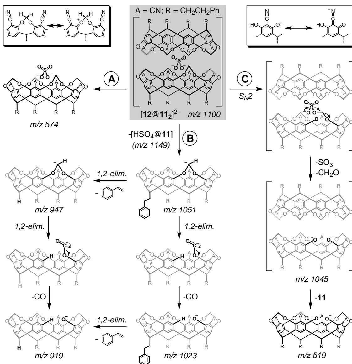
**Scheme S1.** Fragmentation pathways (A, B, C) of [12@11]<sub>2</sub><sup>-</sup> as observed in the CID mass spectra. The insets show the effect of electron-withdrawing substituents such as nitrile on the acetal C-H polarization and the phenolate leaving group properties
