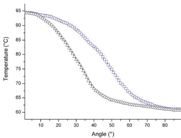
**Supplementary Figure 3.** Temperature transition between the temperature zones 1 and 2 along the traveling path of the droplet extracted from figure 2 and supplementary figure 2c. a) The open triangles show the thermocycling protocol 1. b) The open squares represent the thermocycling protocol 2. A rotation of 90 ° translated into a traveling distance of 5.8 mm.
