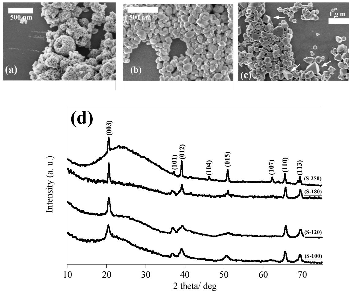
The SEM images show that the self-assembly of the spherical structure was observed with a diameter of several hundred nanometers for the tertiary structure at 120°C. The surface features exhibited similar physical stacking of the nanosized
