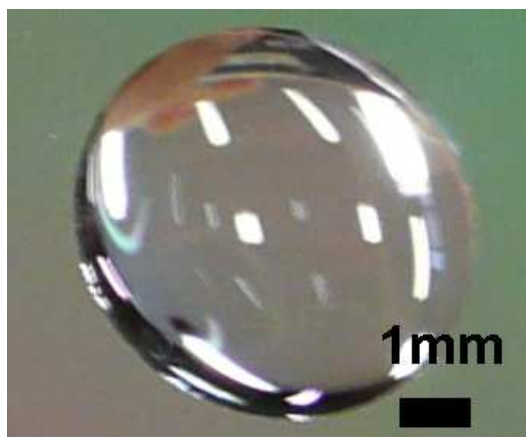
Supporting Figure 3. A cap morphology on a surface consisting of planar silica ( \theta \approx 0^\circ ) and planar fluoropolymer ( \theta \approx 105^\circ ) surfaces. No air bubble gets trapped inside the droplet.
