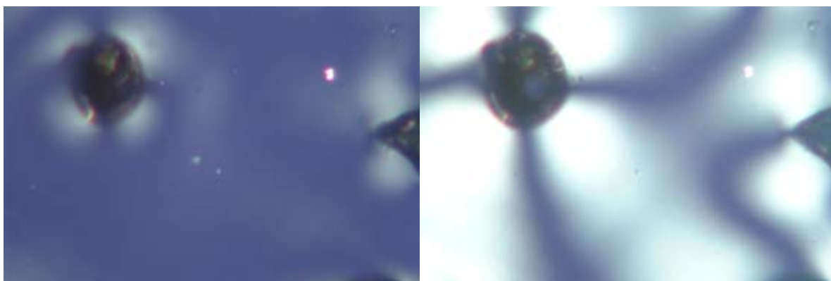
Texture of the cubic phase of 6a obtained upon pressure on the glass-slide (50 °C).
