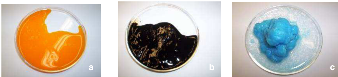
Figure S2. Metal precursors solutions mixed in-situ . (a) Mo-V-Te-Nb-Ox precursor (orange opaque gel), (b) MnOx precursor (brown gel), and (c) CuO/ZnO/Al 2 O 3 precursor (blue gel).
