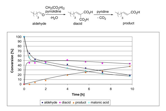
The general method V was used at 10 °C. Trimethoxybenzene (1.66 mmol, 0.33 eq) was added as NMR standard and the conversion was determined by  ${}^{1}$ H-NMR.
