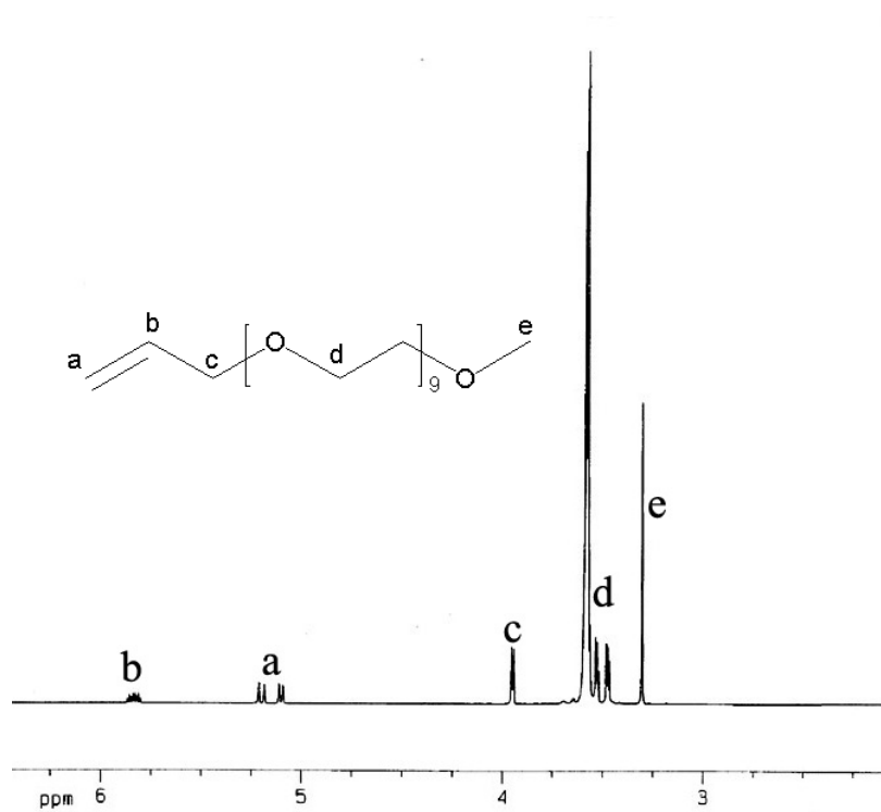
Figure S1. ^1\text{H} -NMR spectrum of PEO 10 in \text{CDCl}_3
